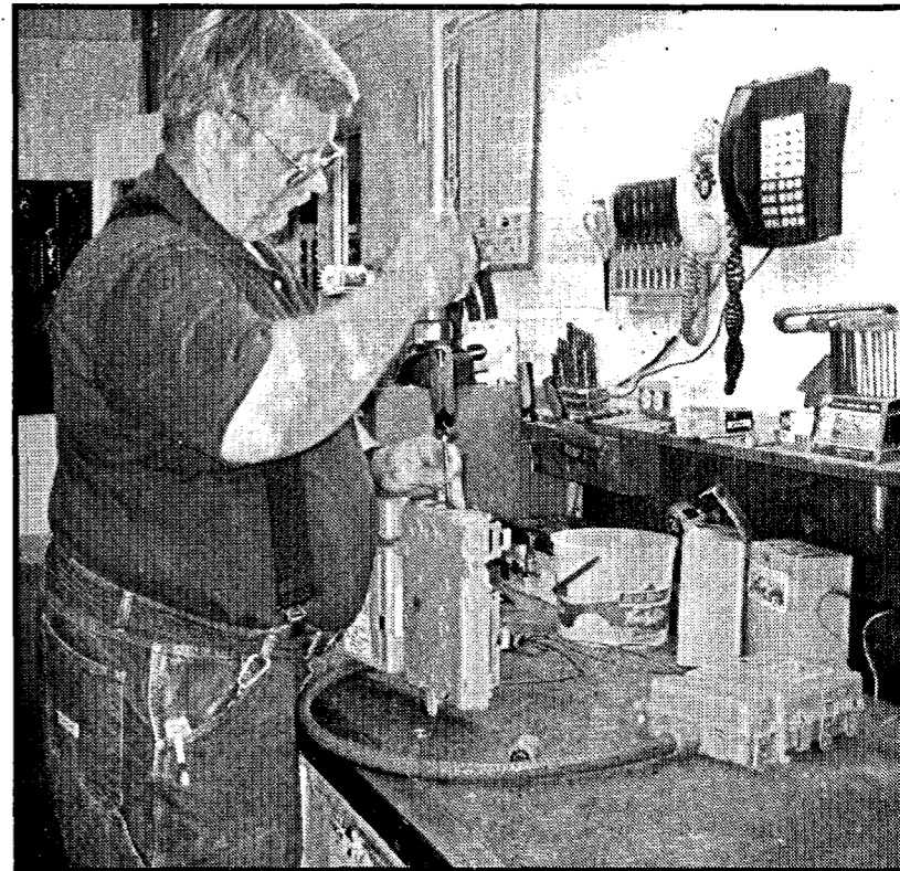
Bill Bretkreutz, an employee with the Wayne Electrical Distribution Department, works on a load control device designed to help conserve electricity.
